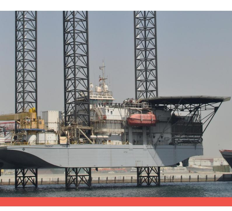
Seafox Trident One is a three-legged, self-elevating, self-propelled jack-up unit for accommodation, well services and platform maintenance support. She was built in 2000 by Arab Heavy Industries in Ajman, UAE. Last conversion took place in 2010.
