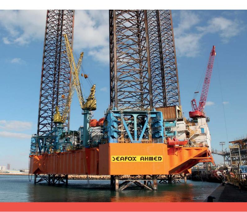
Seafox Ahmed is a three-legged, self-elevating jack-up unit for accommodation and offshore support services built in Vicksburg, Mississippi (USA), by Marathon LeTourneau. She was originally converted to a jack-up ASV in 1993 by Lamprell, in Sharjah, UAE. The last upgrade took place in 2007.
