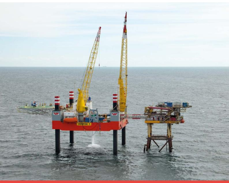
MAIN CRANE CAPACITY 300 t | ACCOMMODATION 75 POB | MAX WATER DEPTH 40 m | DECK SPACE 600 m<sup>2</sup>
