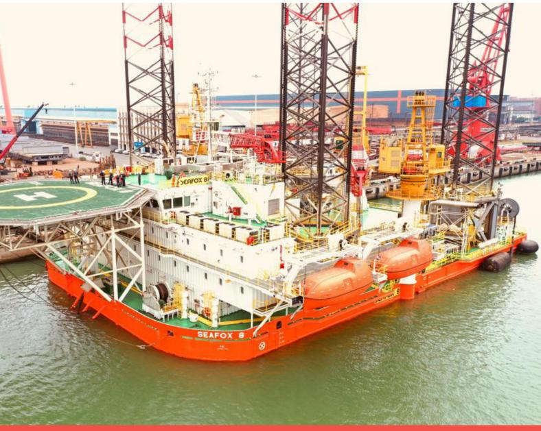
MAIN CRANE CAPACITY 220 t | POB 150 (UPGRADABLE) | MAX WATER DEPTH 85 m | DECK SPACE 1.200 m<sup>2</sup>
