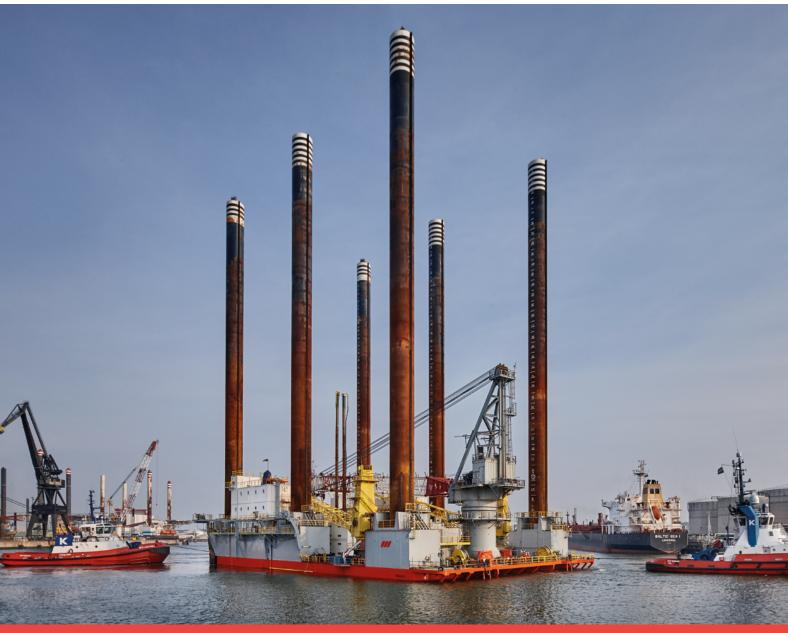
MAIN CRANE CAPACITY 300 t | ACCOMMODATION 153 POB | MAX WATER DEPTH 45 m | DECK SPACE 900 m<sup>2</sup>
