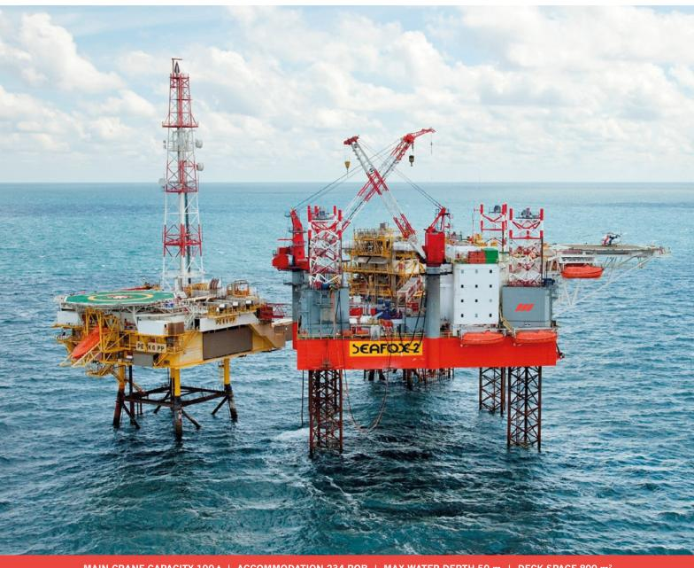
MAIN CRANE CAPACITY 100 t | ACCOMMODATION 234 POB | MAX WATER DEPTH 50 m | DECK SPACE 800 m<sup>2</sup>
